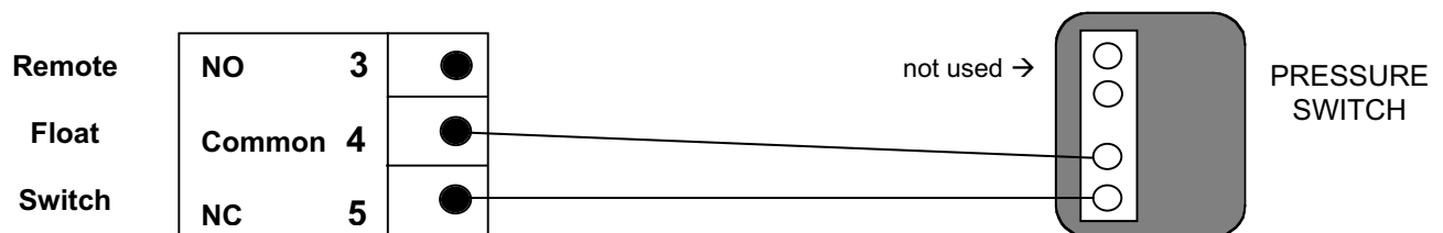
ILLUSTRATION Pressure switch connected to the junction box for “remote switching”
